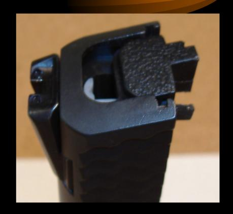
Release striker by pushing down on firing pin block.
