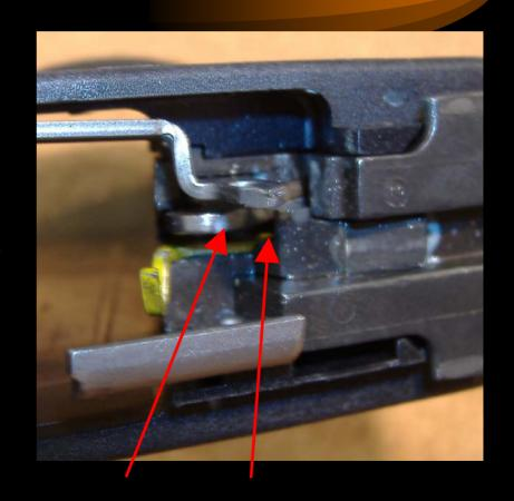
• Use proper size punch to drive rear role pin out of frame.
