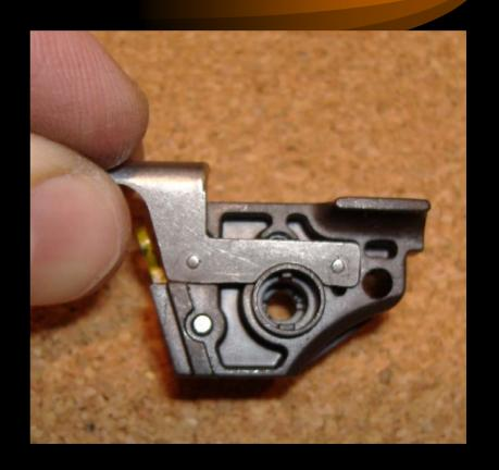
• Slide leg of trigger bar into slot on on sear housing block. It is just below the sear.
