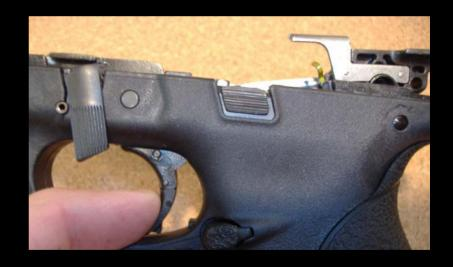
• Once the sear housing block clears the frame, it will slide right off the back of the trigger bar.
