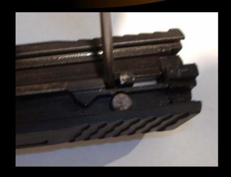
Once striker sleeve is pushed forward, end cap will slide off as shown.
