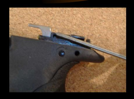
• Once sear housing block starts to come up out of the frame, pull the trigger to take tension off the trigger bar.
